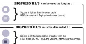
Vaccine Vial Monitors (VVM2) are part of the label on all bOPV 1 & 3 vials. VVM2 are supplied by TEMPTIME Corporation, U.S.A. The colour dot which appears on the label of the vial is a VVM2. This is a time-temperature sensitive dot that provides an indication of the cumulative heat to which the vial has been exposed. It warns the end user when exposure to heat is likely to have degraded the vaccine beyond an acceptable level.
