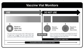
The interpretation of VVM2 is simple. Focus on the central square. Its colour will change progressively. As long as the colour of this square is lighter than the colour of the ring, the vaccine can be used. As soon as the colour of the central square is the same colour as the ring or of a darker colour than the ring, the vial should be
